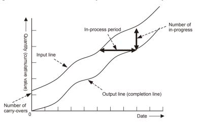
•Figure 5-20 How to Find a Delivery Date from the Fluidity Number Curve
