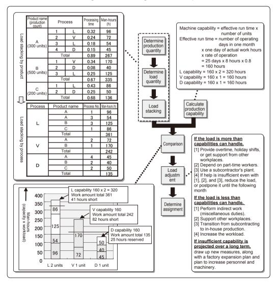
Diagram 5-21 Loading Process Example
